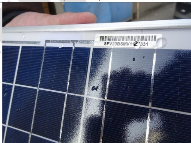
After water-proof test
