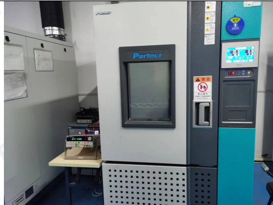
湿热循环架设;Test setup of humid heat cycle
