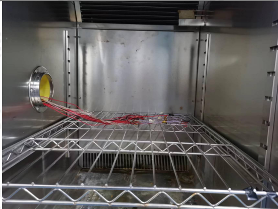
湿热循环架设;Test setup of humid heat cycle
