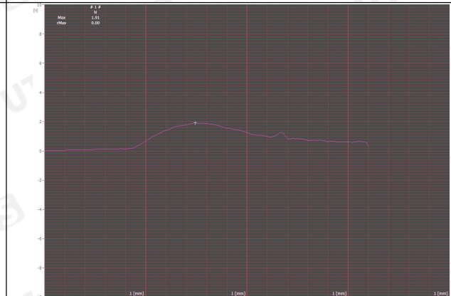
8PIN 插入力; Test curve-8PIN insertion force
