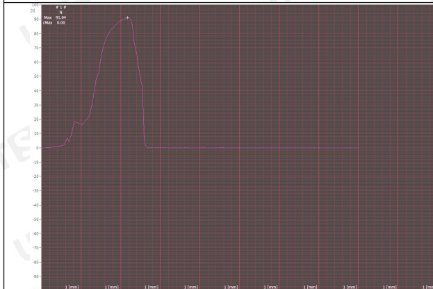
2PIN 2 次锁拔出力; Test curve-2PIN 2nd level lock extraction force
