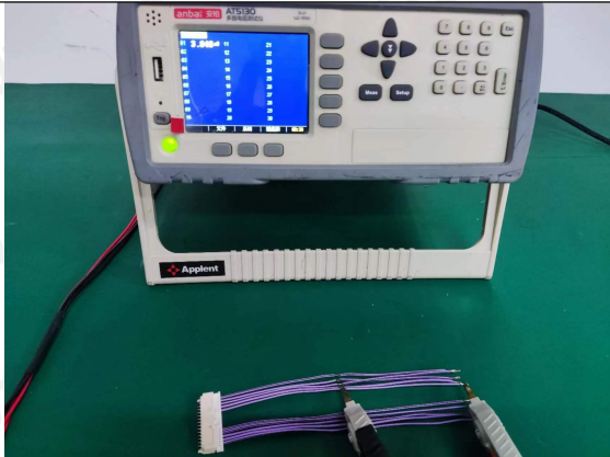
接触电阻(测试后)- Contact resistance (after test)
