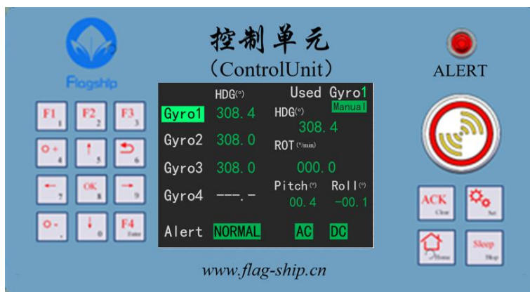
Figure 2-2 Control Unit (CU) Panel
